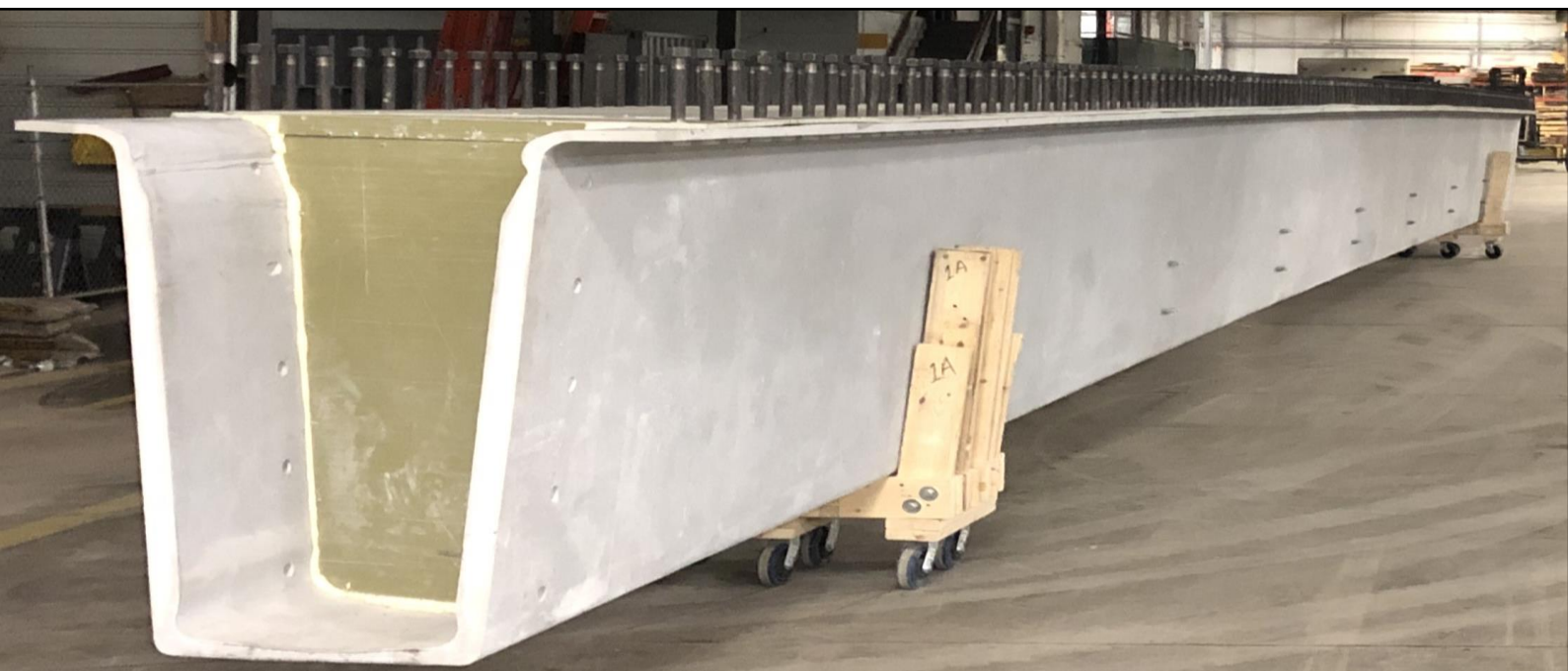
Mold used to make 30'-60' Spans
