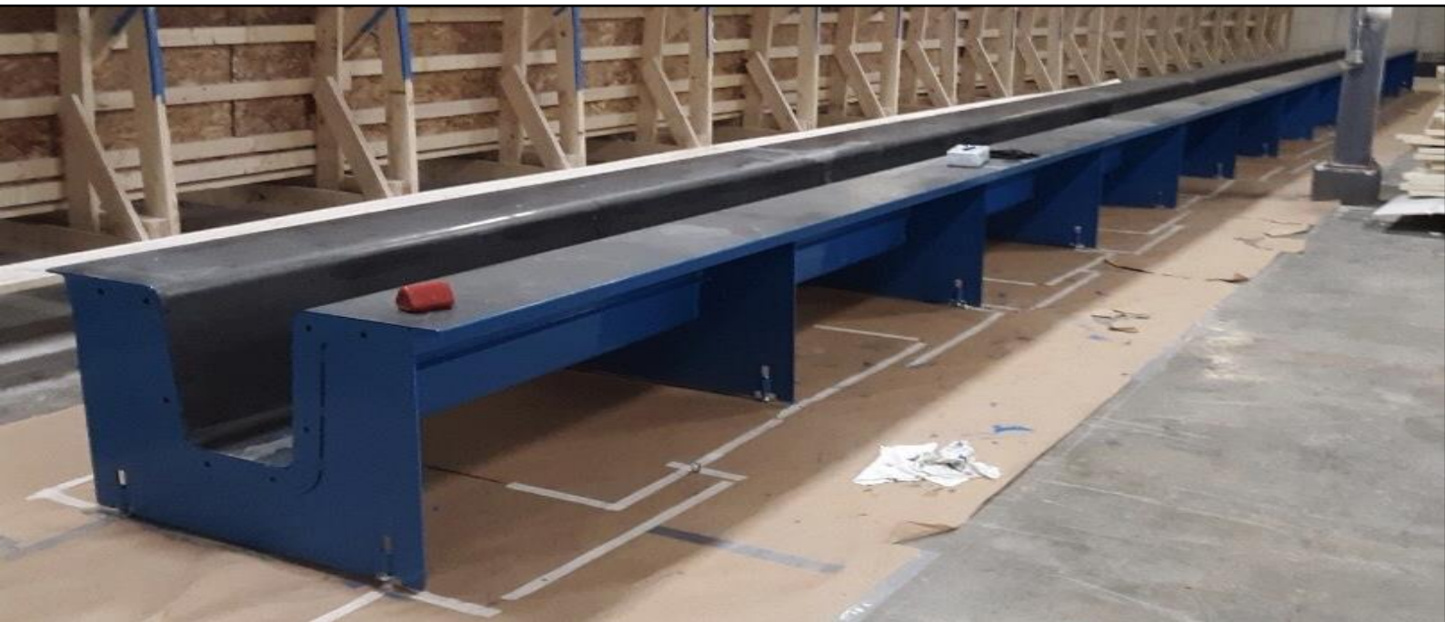
Mold used to make 30'-60' Spans
